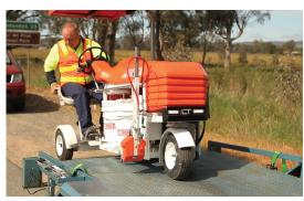
The LineTrike weighs only 347kg (empty) so it can be transported on a single axle trailer. It drives on and off with ease, making set up time and packing up much faster and easier.
